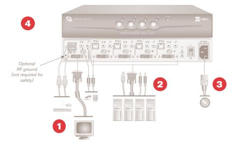
switch. Plug one end into the IEC power connector on the SwitchView SC4 UAD switch. Ensure the power switch is off, then plug the other end of the power cord into an AC wall outlet. Turn on your switch first, then turn on all attached servers.
